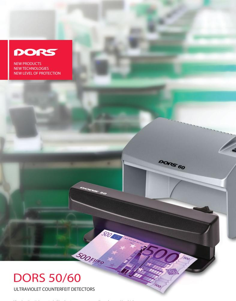
Visual authenticity control of banknotes, passports, credit cards, securities, high security forms and duty stamps by visualizing protective features fluorescent in ultraviolet light.
